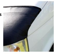
Now attach each of the hooks (on the elastics) to the available fixing points on the under side of the bonnet hood (As pictured to the right)
